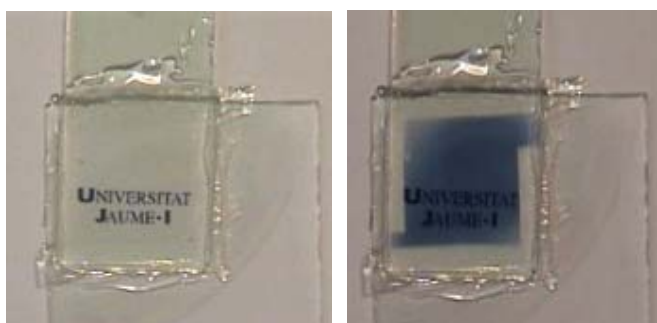
Fig. 7.4. Electrochromic device B (Sb-doped \text{SnO}_2 as counter electrode) in the bleached ( 2.0 \text{ V} , left) and coloured ( -3.0 \text{ V} , right) state. Approximately a 65% transmittance change can be obtained. Area \sim 1 \text{ cm}^2 .
