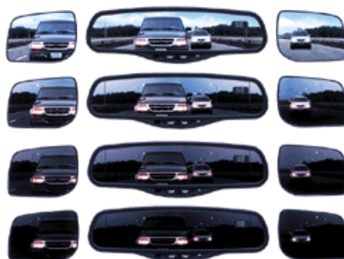
Fig. 1.15. Electrochromic rear-view mirrors developed by Gentex ( www.gentex.com ).
