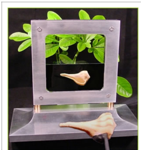
Fig. 1.12. Switchable mirror prototype showing transparent (above) and reflective (below) states.
