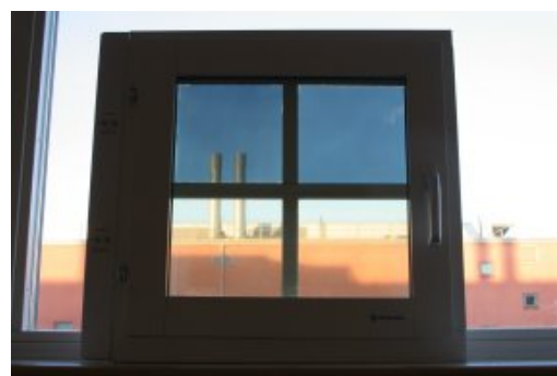
Fig. 1.11. Electrochromic window using \text{WO}_3 as electrochromic material.
