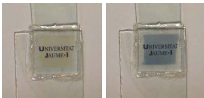
Fig. 7.3. Electrochromic device A (PEDOP as counter electrode) in the bleached ( 2.2 \text{ V} , left) and coloured ( -3.2 \text{ V} , right) state. Approximately a 40% transmittance change can be obtained. Area \sim 1 \text{ cm}^2 .
