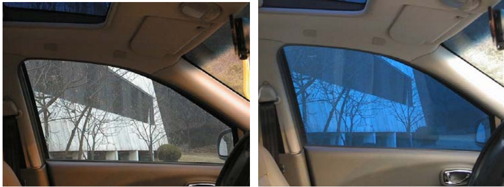
Fig. 1.9. Suspended particle device (SPD) car window by Research Frontiers Incorporated. Transparent (on-state) on the left and colored (off-state) on the right.
