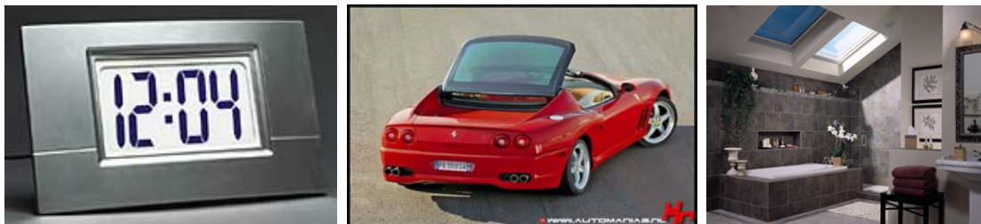
Fig. 1.16. Electrochromic displays by NTERA (left) offer an ink-on-paper readability at a competitive cost. In the middle, the electrochromic sunroof used in Ferrari Superamerica developed by Saint-Gobain. It changes from clear to almost black in about 60 seconds. Electrochromic SageGlass skylights are on the right.
