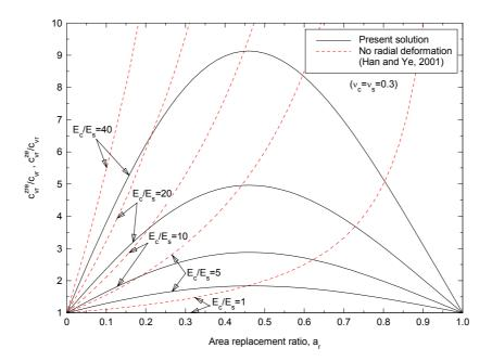
For high replacement ratios, Han and Ye propose a high equivalent consolidation coefficient to compensate the large initial settlement that is not included in their solution.
