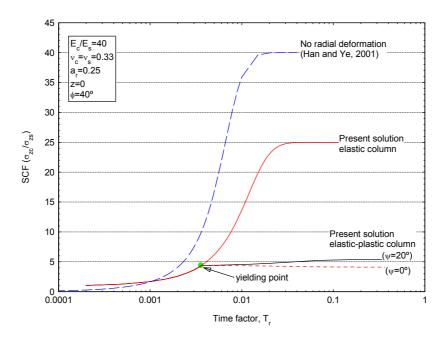
The stress concentration ratio decreases by nearly a half if radial strains of the column are considered, but yielding of the column is needed to get realistic values.
