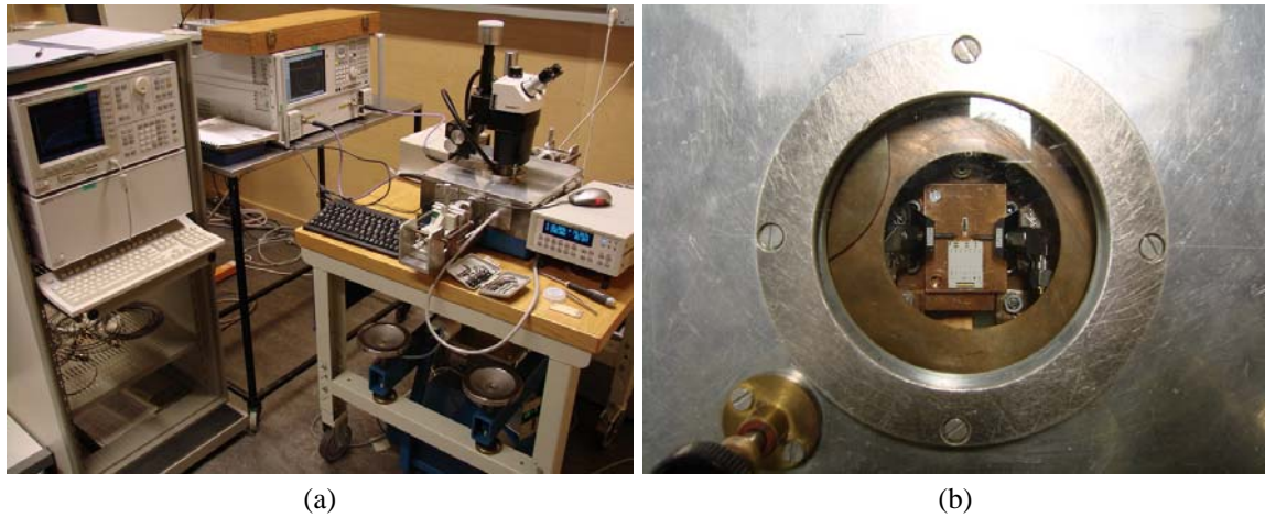
Fig. 4.3. Pictures of the measurement setup; (a) general view of the setup; (b) detailed view through the Dewar window of some transistors together with the calibration substrate.
