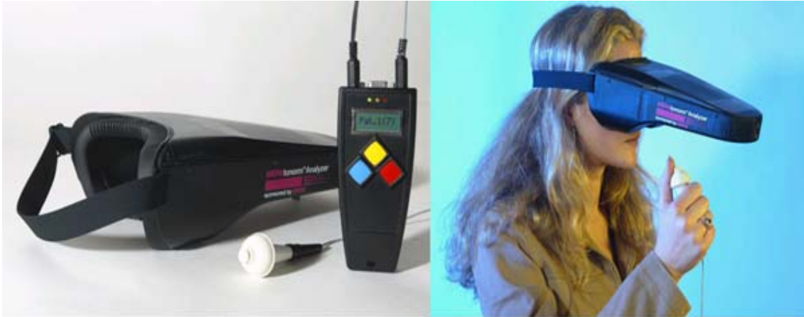
Fig.5. Critical Flicker Frequency (CFF). Sistema comercial Hepatonorm Analyzer R
