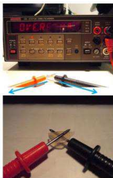
Figure 4.25. Intrinsic electrical conductivity measurement by sensitive ohm meter
