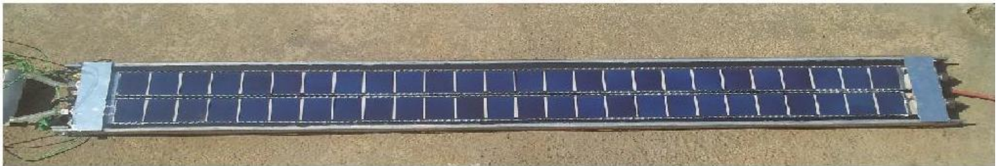
Figure 35. The CPV modules: designed and assembled at the applied physics laboratory at the University of Lleida (Spain)
