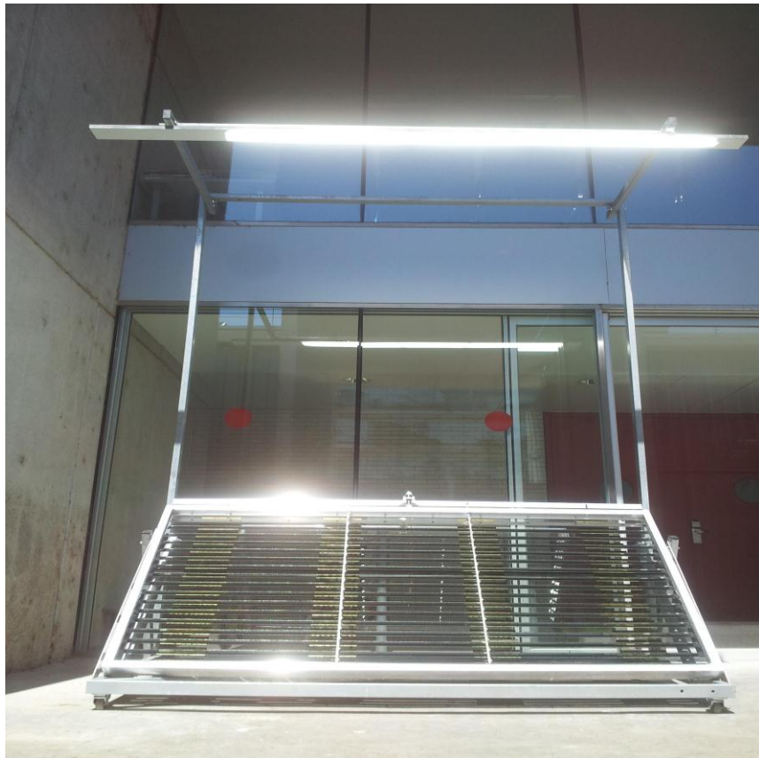
Figure 36. The concentration system used: Assembled at the applied physics laboratory at the University of Lleida (Spain)
