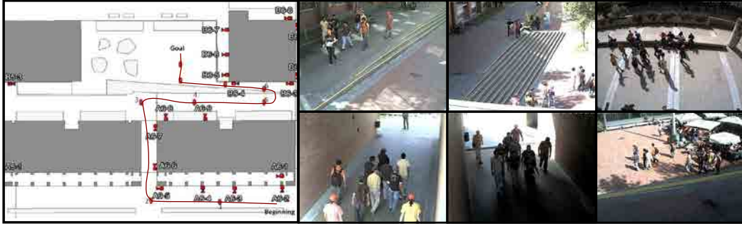
Figure 4.7: Barcelona Robot Lab. Left: An aerial view of our experimental site, the Barcelona Robot Lab, and the distribution of cameras in the network. The solid line depicts a sample path followed by the group of persons and guides. Right: A few images of the group of people, seen from different cameras.
