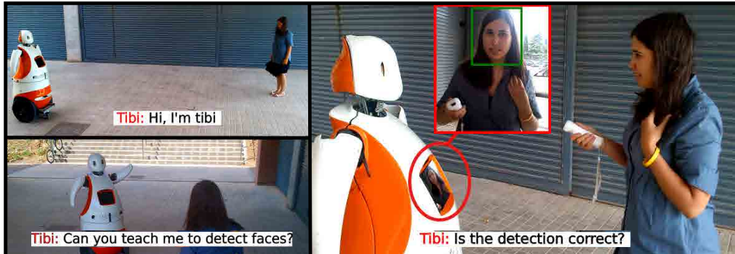
Figure 6.1: Human-Robot Interaction and Communication. Left: Tibi mobile robot approaches a person to initiate a conversation. Right: After the first contact, the person assists Tibi to improve its visual skills. A Wii's remote controller is used to help to validate and improve the visual detector.
