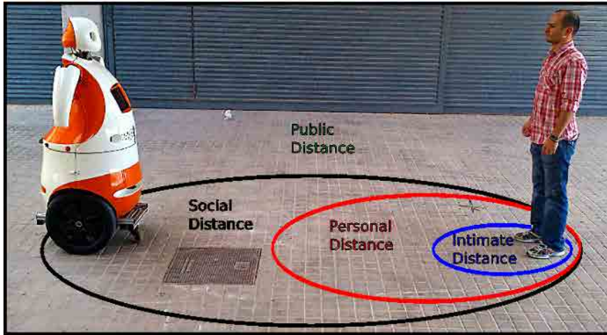
Figure 6.3: Levels of Engagement. Robot-to-person levels of distance, to distinguish levels of engagement while interacting.
