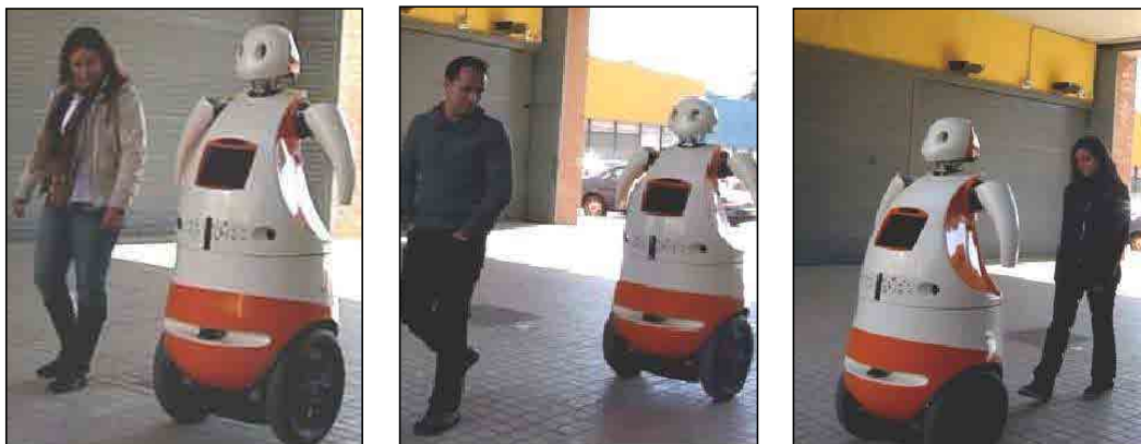
Figure 5.6: People walking with Tibi Robot. Left: Tibi walks side by side with the volunteer. Center: Robot walks behind the person pushing him/her (the Helblings' pushing force is applied). Right: Tibi walks in front the person and, here, the dragging force is applied.
