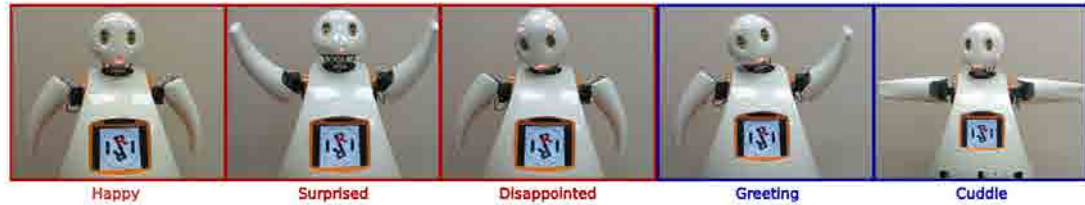
Figure 6.5: Tibi Gestures. Movements performed by Tibi during experiments. Left: Three different emotional expressions. Right: Two actions.
