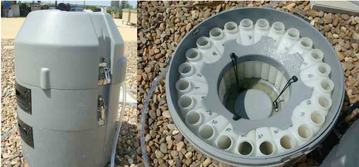
Figure 7.3. View of the autosamplers (left) and the 24 bottles (right) used for water sampling at the different units of the pilot hybrid treatment system.
