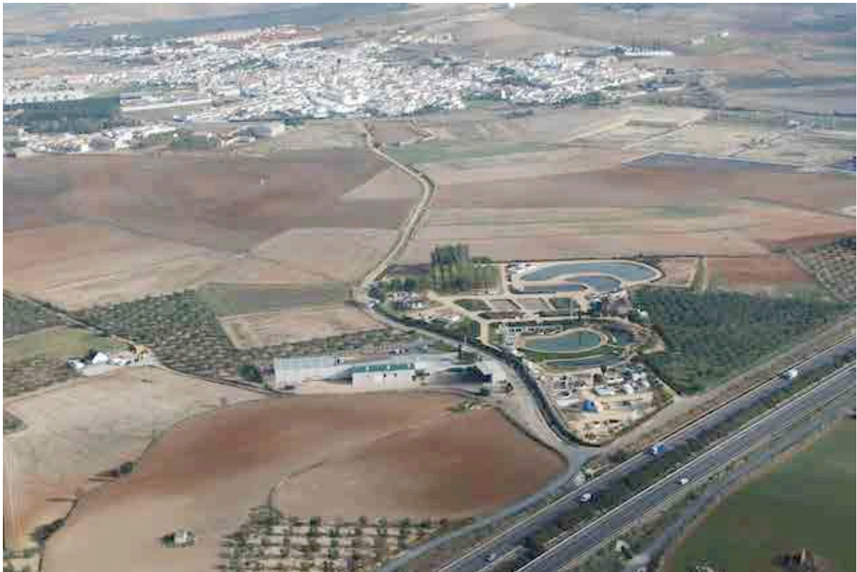
Figure 8.2. Aerial view of the 41000-m 2 pilot-scale experimental treatment facility of the Foundation Centre for New Water Technologies (CENTA) located Carrión de los Céspedes (2300 PE), south Spain.
