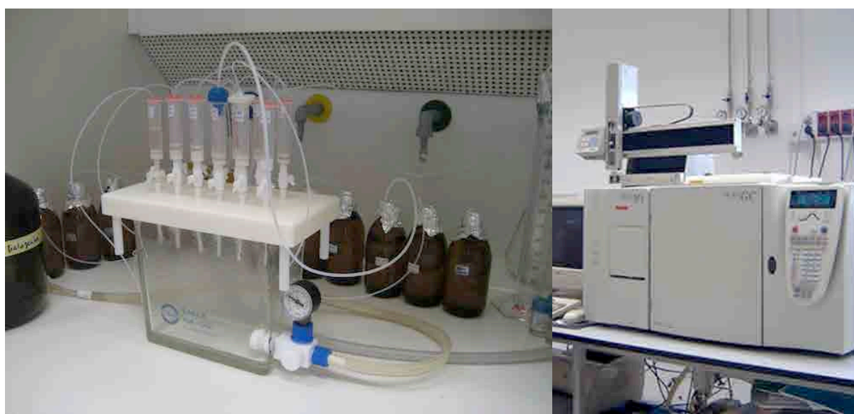
Figure 3.3. View of the solid phase extraction and the GC-MS equipment used for the determination of target emerging organic contaminants.
