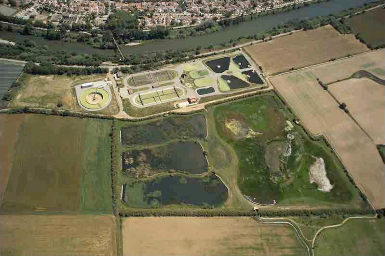
Figure 1.3. Aerial view of the activated sludge WWTP and tertiary treatment constructed wetland system at the Natural Park of Aiguamolls de l'Empordà, Girona, Spain (photo: Consorci Costa Brava).
