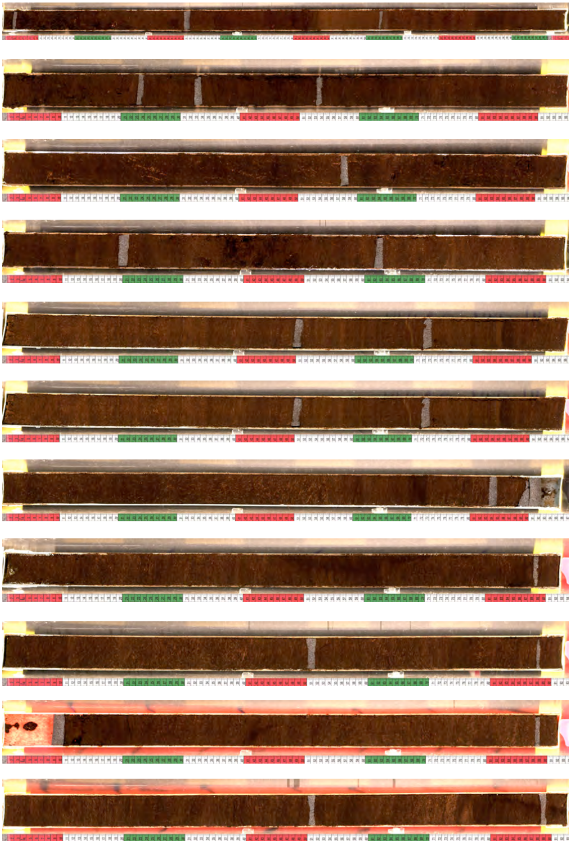
Figure 3. 3. Images acquired from (up to down) ARO 06 01 section 01, 02, 03, 04, 05, 06, 07, 08, 09, 10, 11 with a line-scan camera. Foam was used to cover missing material sampled for radiocarbon dating.
