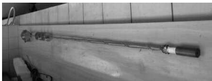
Figure 4.3: View of the probe with the differential scanning calorimeter (copper spool) at the right-hand side, adapted to be used with the Teslatron cryomagnetic system.
