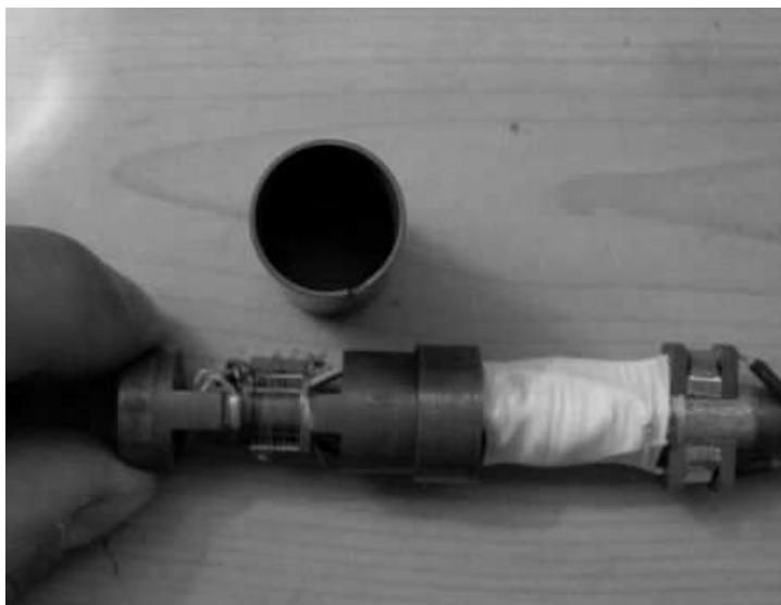
Figure 4.4: Detail of the differential scanning calorimeter.
