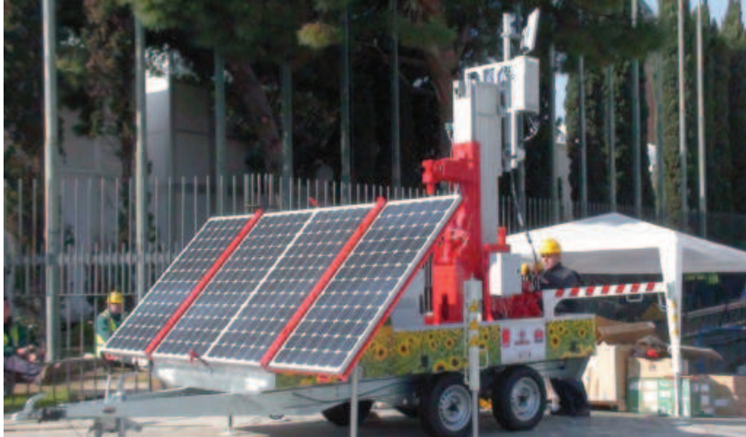
Figure 2.5: Base station entirely powered with solar energy, which was used in the 2010 Mobile World Congress in Barcelona [34].
