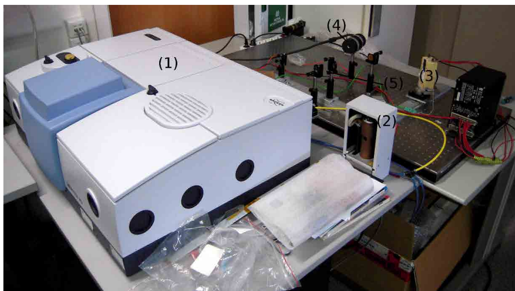
Figure B.1: Temperature characterization setup: (1) FTIR; (2) low-temperature heater; (3) high-temperature heater; (4) BB; (5) optical path.
