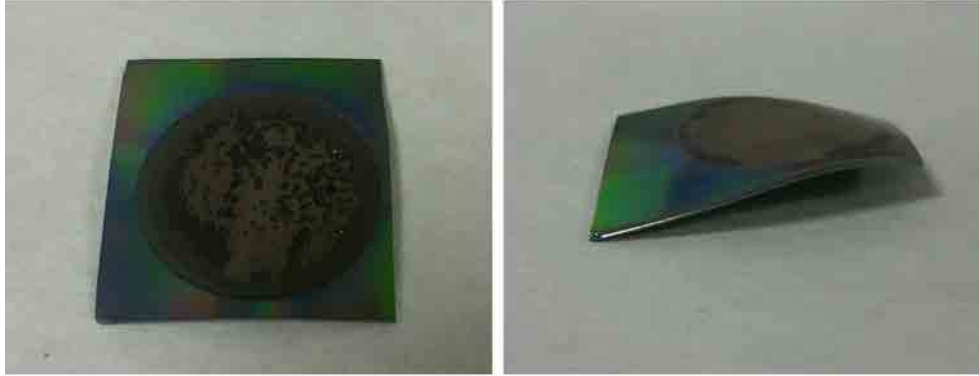
Figure 5.10: Degradation suffered by ALD-coated sample after 8 hours at 1200 K in air atmosphere.
