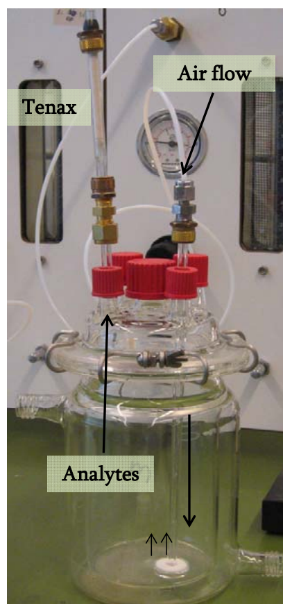
Figure 1. Schematic picture of the extraction assembly carried out in the sample extraction procedure indicating the air flow entrance which pushes the analytes from the gas phase present inside the system towards the exit with the Tenax trap set-up
