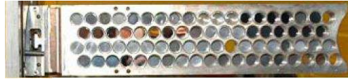
Figure 2.4: Picture of the 72 production targets at the entrance of the FRS with its support. The optimum target can be selected remotely.
