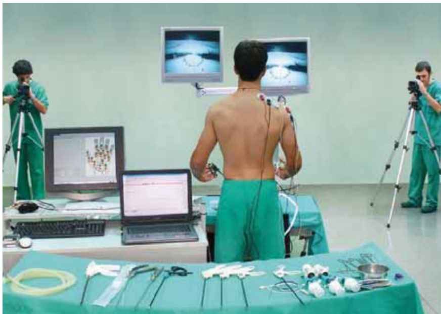
Figure 5. Detail of the ergonomic study. The surface electromyography is combined with three-dimensional video-analysis.
