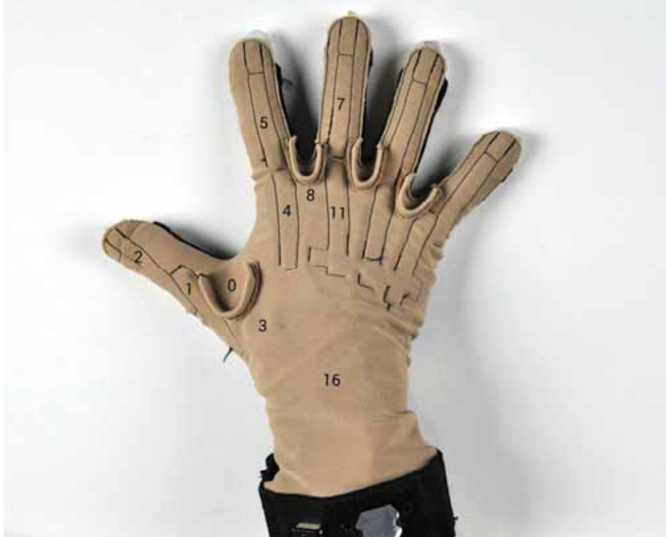
Figure 5. Position of each sensor on the surgeon's hand and wrist. 264x213mm (300 x 300 DPI)
