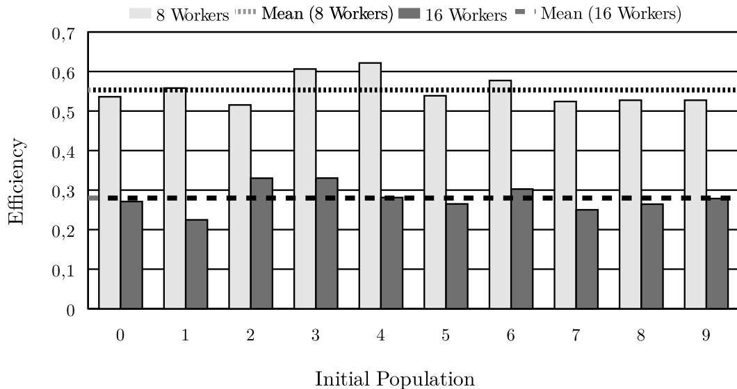
Figure 2.14: Efficiency obtained for 10 different executions of the GA with TAC and the efficient TAC.
