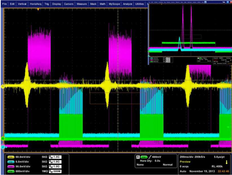
FIGURE 4.14: Oscilloscope trace of a typical experimental sequence (200 ms/div). Yellow: Cryostat pulses, generated directly by the piezoelectric element. Each pulse is composed of 17 kHz oscillations. Purple: Memory preparation and control pulses. Blue: series of input pulses to be stored in the memory and green: Trigger signal created by the AWG for individual storage trial. Inset (5 \mu s/div): zoomed view to show individual input pulse, trigger and the pair of control pulses.
