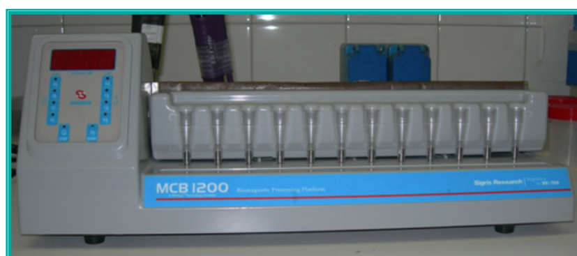
Figure 3.8. MCB 1200 biomagnetic processing platform in which magnetic separations are carried out.
