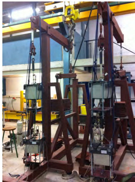
Figure B.2: FRP pull-outs under sustained loads.
