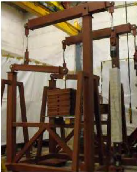
Figure A.1: Frames for long-term tensile tests.
