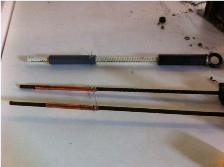
Figure B.4: Reinforcing bars previous to cast (bond length being already defined).
