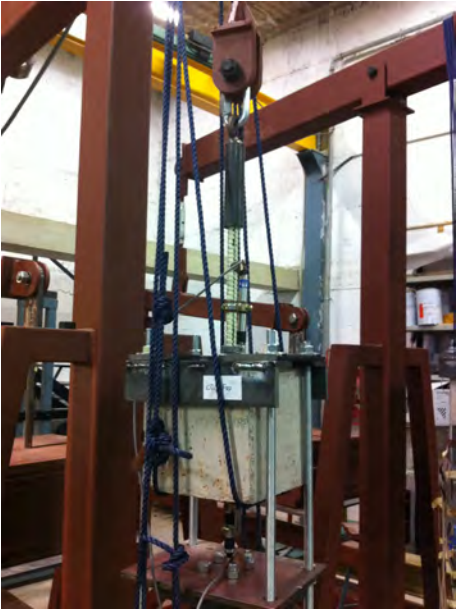
Figure B.7: Pull-out instrumentation during testing.
