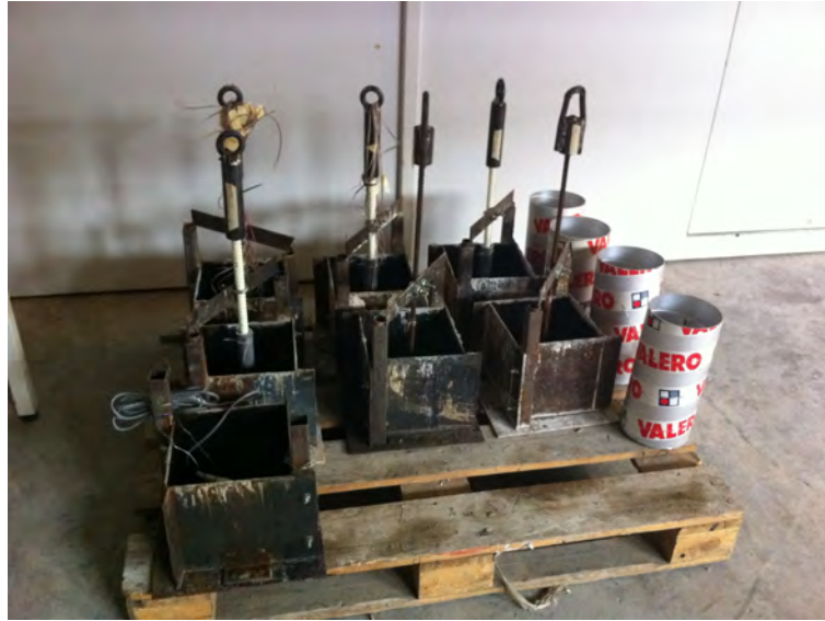
Figure B.5: Moulds for pull-out specimens' casting.
