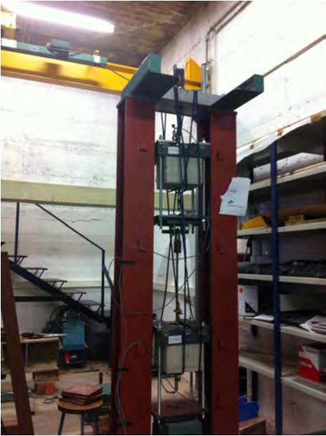
Figure B.3: Steel pull-outs under sustained loads.
