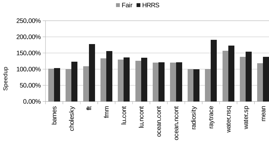
Figure 5.8: Speedup comparison of the HRRS and Fairness scheduler normalized to Linux OS scheduler for the SPLASH-2 benchmark suite running on four cores (1 OoO + 3 InO)
