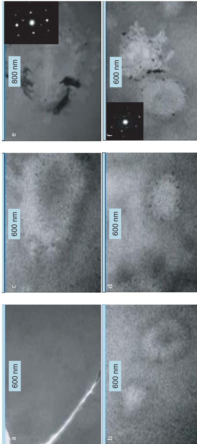
Fig. 4.7: Illustration of crystallization behavior in-situ - annealing in the supercooled liquid region (723K) (K 260-5): (a) is the initial microstructure, before annealing; (b)-(c)-(d) phase segregation observed during minute 1; (e)-(f) crystals formed out of the white areas after 10 minutes of holding with their respective diffraction patterns given in the insets.
