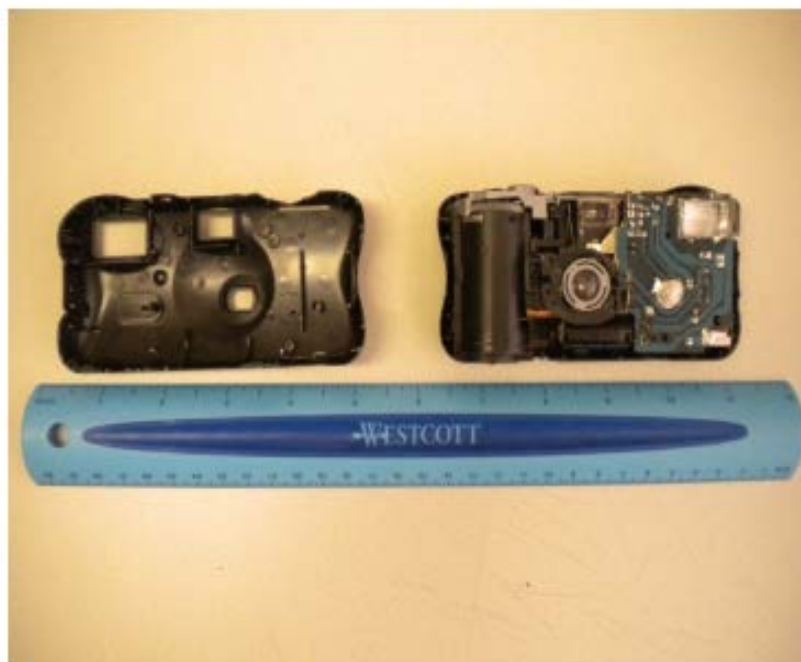
Figure 7.8 Exploded view II of a Dissected Kodak Flash Camera, [Edwards et al. 2010]
