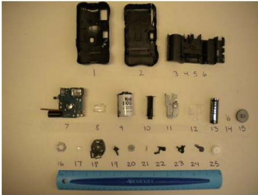
Figure 7.7 Exploded view I of a Dissected Kodak Flash Camera, [Edwards et al. 2010]
