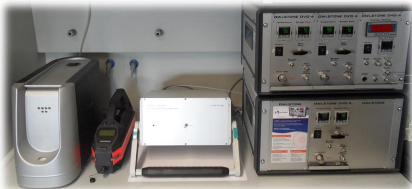
Figure 3.2 The OVG calibration gas generator developed by Owlstone (Owlstone, 2014) together with IMS used in this present thesis
