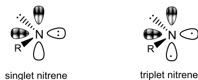
Figure 3.2. Electronic structure of triplet and singlet nitrenes
