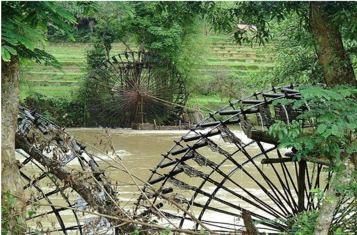
Photo 39. Traditional water wheels collectively made by villagers from local resources mainly bamboos and small woods that villagers withdraw from within CPR system inside their village territory Source: http://www.visit-viengxay.com
