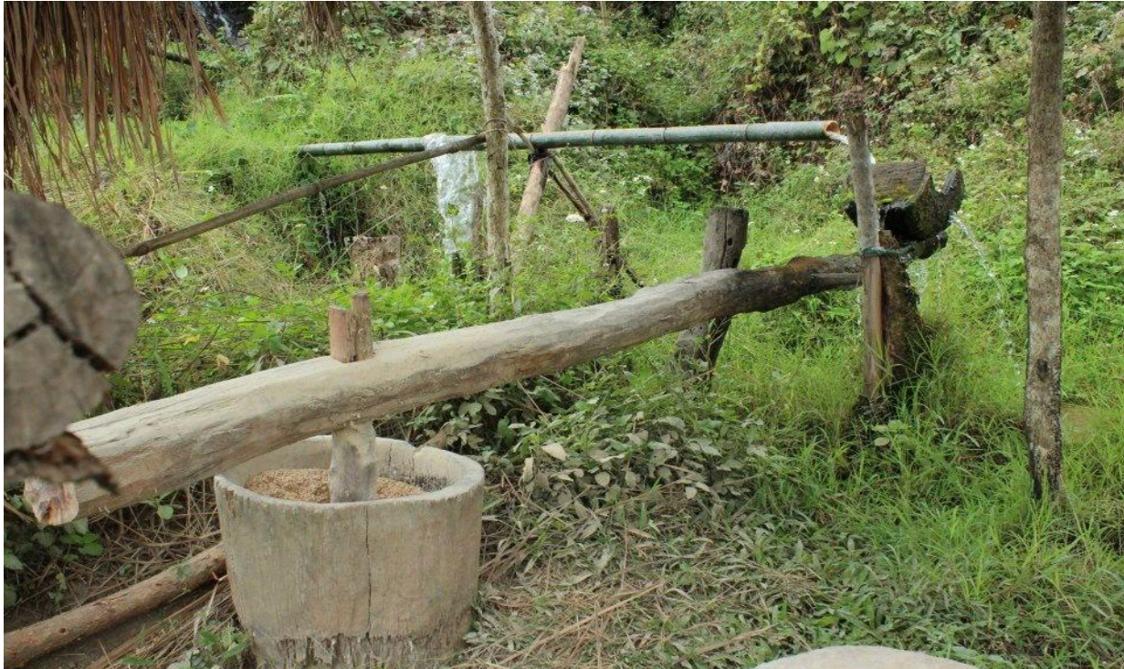
Photo 50. Before an introduction of new technology, villagers used traditional rice mill that used energy from the flow in streams to pound rice. It was located near a river or stream outside the residential area and processing crops through this traditional method was woman's responsibility. Source: www.google.com .
