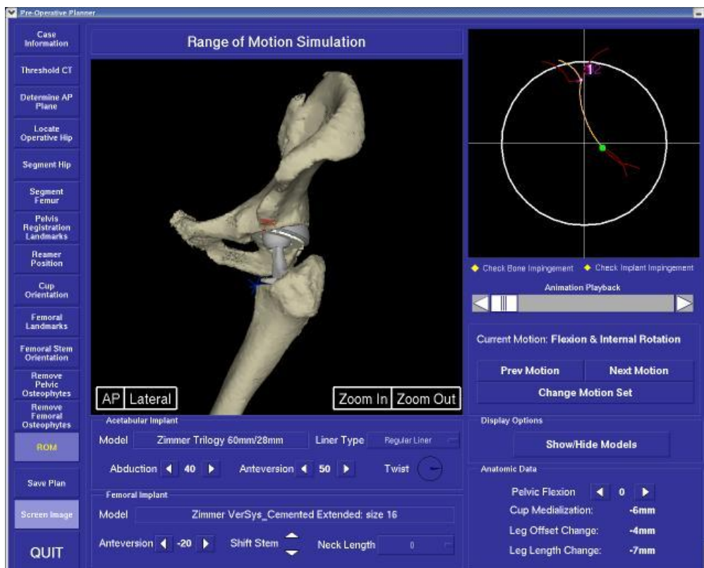
Fig.1: A screenshot image of the HipNav® navigation screen which shows the importance of correct combined anteversion. For any one given motion path (flexion, extension, internal rotation, etc) the implant positions influence the range of motion to impingement and thus risk for dislocation, wear and loosening.
