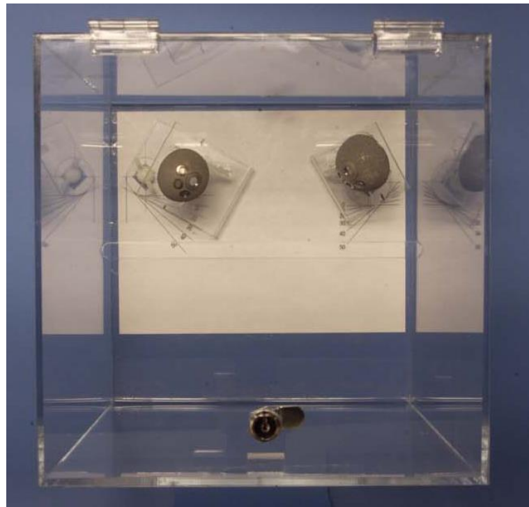
Fig. 1 A and B: The phantom model is a symmetrical silicone cube incorporating embedded markers for the APP and 2 calibrated acetabular implants that represent the right and left hips, respectively. The cube is constructed to scale to represent an anatomic pelvic with 2 prosthetic acetabulae implanted in each hip. The superior view of the phantom cube illustrates the acetabular position marked by angle measurement references on a protractor.
