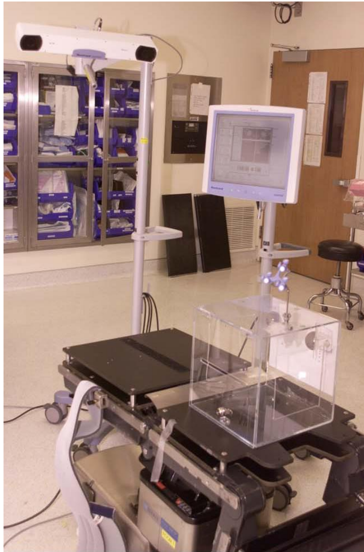
Fig 5 A: The setup of the operating room with the phantom model and the Navitrack Imageless Navigation System with its sensor and display screen. A rigid tracking device used to reference acetabular cup positions during registration is shown. The setup is equivalent to the clinically navigated cup in a patient during surgery.
