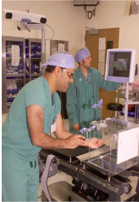
Fig 5 B: Registration process with the pointer to measure the acetabular cups position similar to a surgical procedure with readings obtained for each cup position (non adjusted anatomic plane and adjusted for tilt coronal plane) displayed on the screen..
