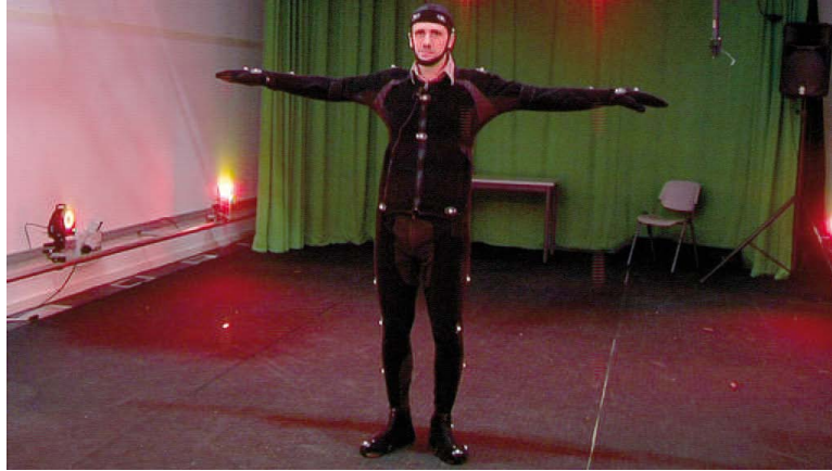
FIGURE 26: SET-UP OF THE RECORDING SESSION. AN OPTICAL MOTION CAPTURE SYSTEM WITH 24 INFRA-RED CAMERAS, A CLIP-ON WIRELESS MICROPHONE, AND A VIDEO CAMERA (NOT IN THE IMAGE). THE ACTOR IS WEARING A BLACK MOTION CAPTURE SUIT WITH REFLECTIVE MARKERS.
