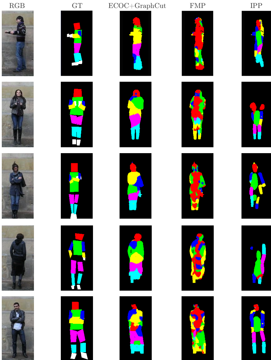
Figure 6.5: Multi-limb segmentation results for the three methods, for each sample, we also show the RGB image and the ground-truth (GT).
