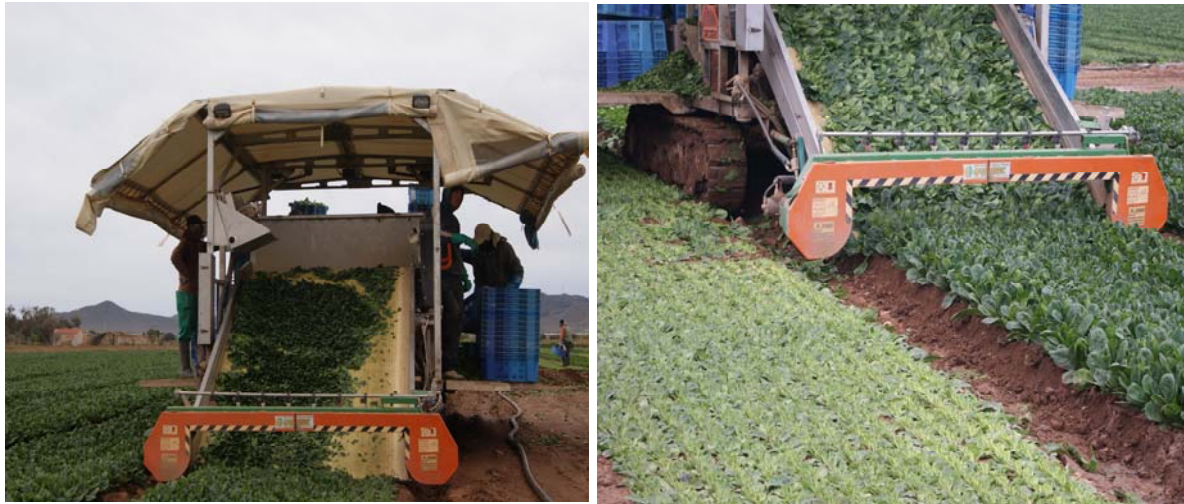
Picture 1.2. (A) Mechanical harvesting of baby spinach. (B) Detailed picture of the conveyor belt of a commercial harvesting machine.
