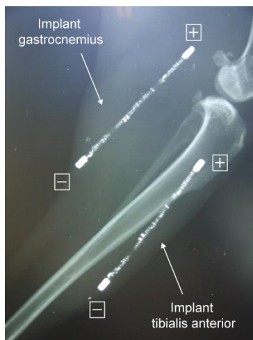
Figure 5.15. X-ray images of the stimulators implanted in the tibialis anterior and gastrocnemius muscles. The '+' and '-' signs denote the positive and negative terminals of the stimulators.
