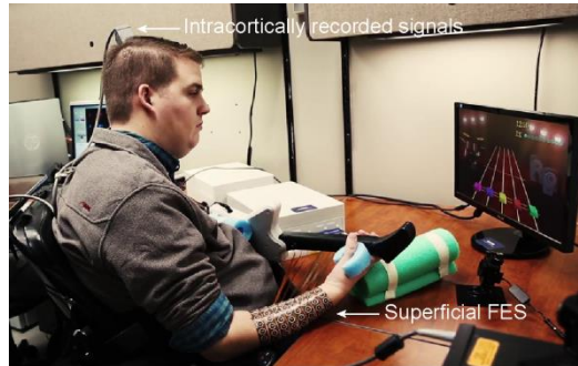
Figure 1.13. Patient playing Guitar Hero by controlling a superficial neuromuscular stimulator using real-time intracortically recorded signals. This system could be greatly improved using a network of wireless implantable microstimulators. Extracted from [113].
