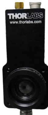
Figure 2.5. . Photomultiplier tube model PMM01 from Thorlabs, Inc. Courtesy of Y. Jauregui Sánchez.
