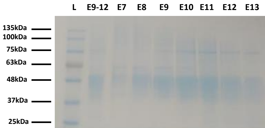
Figure 4.6.3.2 Stained SDS-PAGE at 12% with comassie blue. Eluted samples from the SEC were loaded in the gel. E9-12 lane represents the concentrated sample before injecting in SEC. Eluted fractions (E7-13) are loaded from lower elution volumes (left) to higher elution volumes (right). Same volume was loaded for all the samples and all are buffered with 20mM Tris-HCl at pH 7.6 and 150mM KCl.
