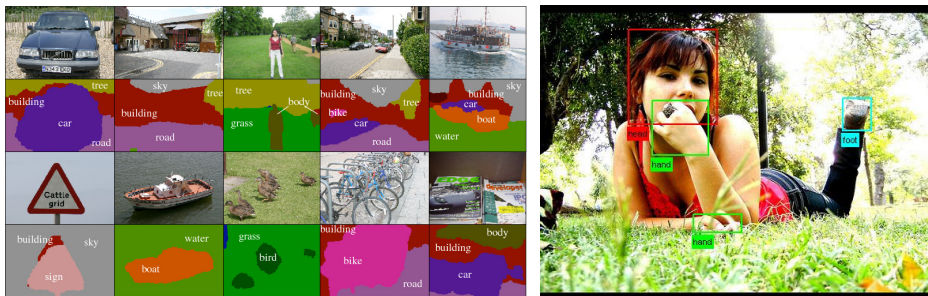
Figure 1.7: Illustration of two classic Computer Vision problems which have been previously addressed using weakly-supervised approaches. Left: Image Semantic Segmentation ( images extracted from the MRSC v2 dataset [Shotton et al., 2006]). Right: Object Detection (examples obtained from the PASCAL VOC2011 Database [Everingham et al., 2015])
