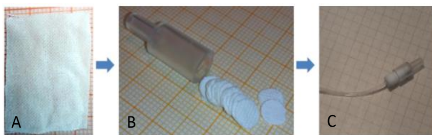
Figure 8. (A) FPSE material; (B) preparation of the minicolumn with FPSE disk; (C) FPSE with minicolumn ready for experiment [188].
