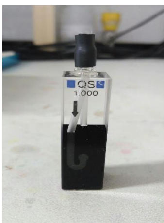
Figure 4.8 Tubing cuvettes which has the inlet and outlet connected via tubes from the cartridge to waste container and located inside the UV spectrophotometer.
