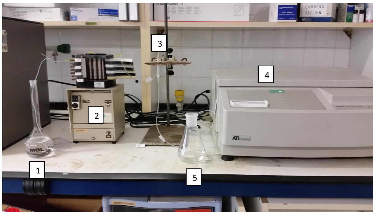
Figure 4.6 Experimental set-up for continuous-flow mode combined with MIP packed cartridge via spectrophotometry detection. 1: standard solution or sample, 2: peristaltic pump, 3: cartridge contained with 10 mg MIP, 4: spectrophotometer, 5: waste container.
