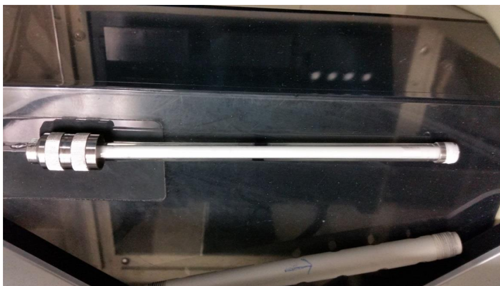
Figure 4.18 Successful MIP-DCF packed in the glass column with inner diameter 3 mm and 15 cm long.
