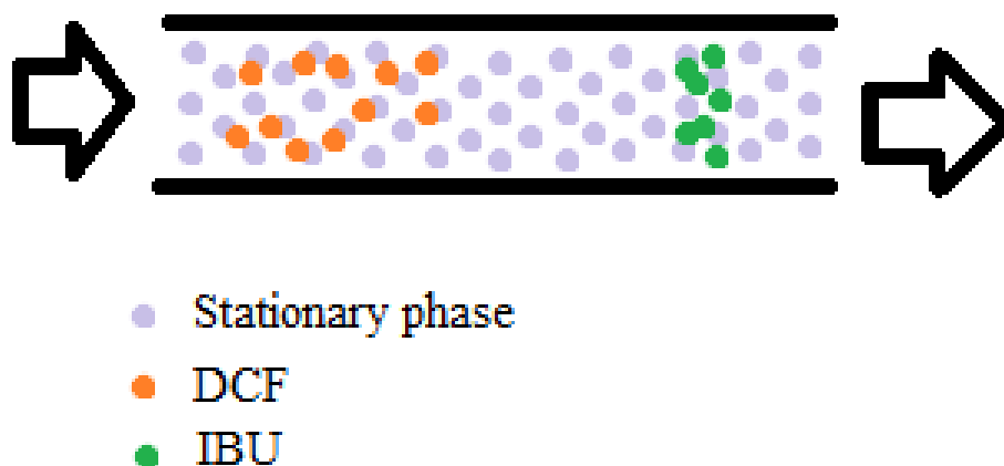
Figure 4.27 DCF molecules tends to remain longer in the column compared to IBU due to the strong hydrogen bonding between MIP-DCF and DCF molecules.
