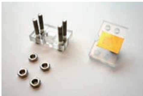
Figure 2.7 Milled methacrylate pieces for micro fuel cell packaging.
