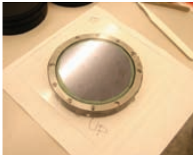
Figure 7.4 Metallic ring used for replication of PDMS master. The picture shows the wafer inside the ring, filled with PDMS and covered by the polycarbonate plate.
