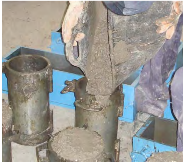
Fig.3.21 - Casting method applied on the manufacturing of the specimens.
