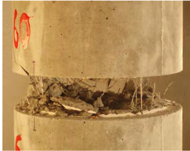
Fig. 3.12 - Final stage of the uniaxial tension test in a specimen from serie A60.
