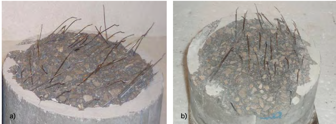
Fig.3.20 - Preferential alignment of fibers at the two cracked surfaces of specimen B60-4: a) Perspective of the out-of-plane; b) Perspective of the in-plane.
