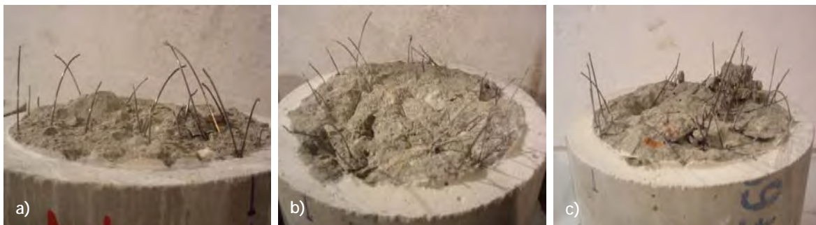
Fig.8.9 - Counting of fibers at one side of the cracked section: a) 20 kg/m 3 ; b) 40 kg/m 3 ; c) 60 kg/m 3 .
