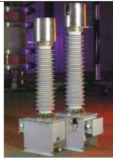
Figure 1.11. 72kV to 145kV single core, single coil magnetic voltage transformer. Insulation of Paper-Oil and a porcelain insulator. Courtesy of Alstom.
