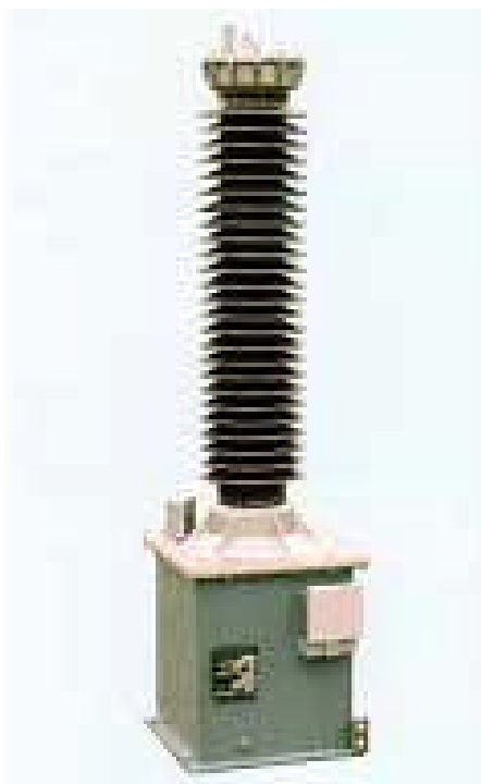
Figure 1.17. Capacitor Voltage Transformer with insulation of film-oil and external porcelain insulator. It is designed by stacking capacitors and incorporates a magnetic VT in the output. Voltage range : 72kV to 765kV. Courtesy of Alstom.
