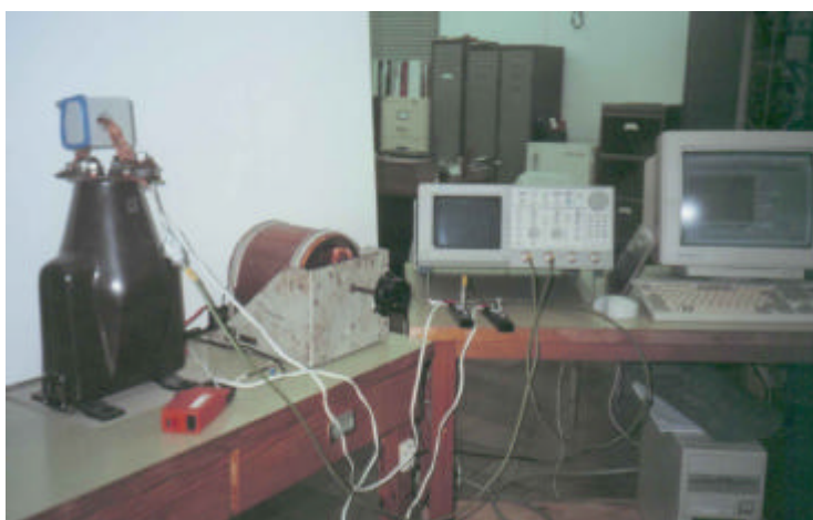
Figure 9.7. Experimental set-up used for testing the Two-Wires Current Sensor
