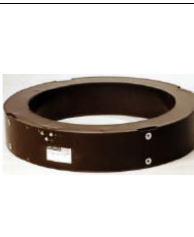
Figure 1.14. Current transformer in cast resin design for high voltage insulation up to 36kV and current rating up to 15000A. Courtesy of Piffner Instrument Transformer, Ltd.
