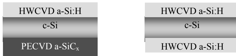
Figure 5.1: Diagram of the two precursors used in this work: with a back a-SiC x passivating layer deposited by PECVD (left) and bifacial precursor with the same layer on both sides (right).
