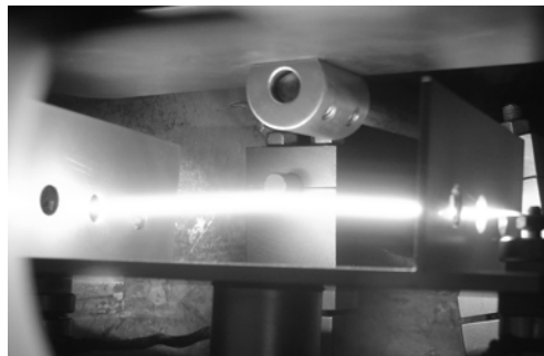
Figure 2.10: Tantalum wire during a HWCVD process.
