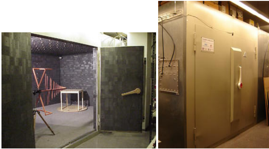
Figure 5.2: Anechoic chamber at UPC premises. This chamber was used due to its good temperature stability and to avoid disturbances during the test (such as people passing by, interferences, etc.).
