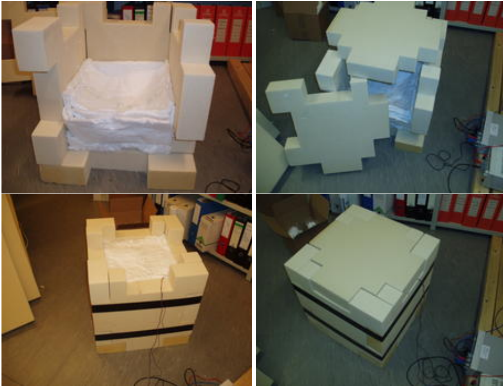
Figure E.2: Construction of the insulator.
