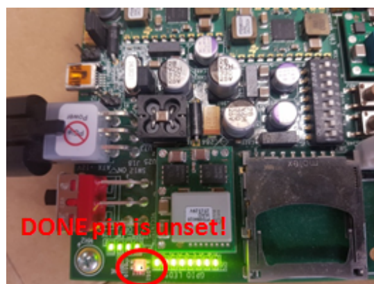
(b) Below the minimum Idle voltage level, i.e. , V_{idleMin} .
