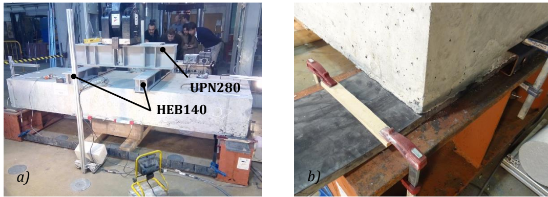
Figure 5.5 a) General configuration of the test and b) neoprene support.
