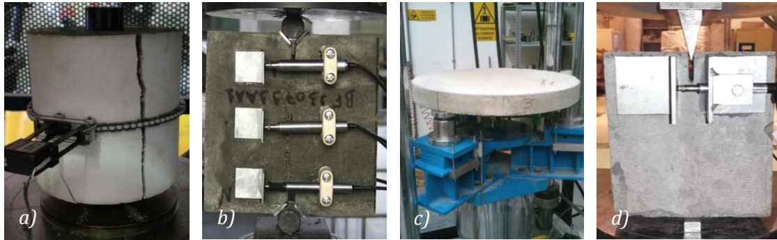
Figure 2.2 a) Barcelona test, b) DEWS (Nunes et al. 2017), c) SRDP (Conforti et al. 2018) and d) Montevideo test (Segura-Castillo et al. 2018b).
