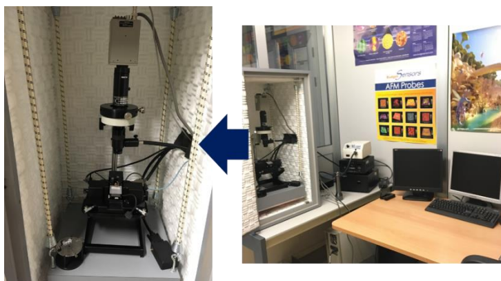
Figure 3.15 Experimental setup for atomic force microscopy measurements
