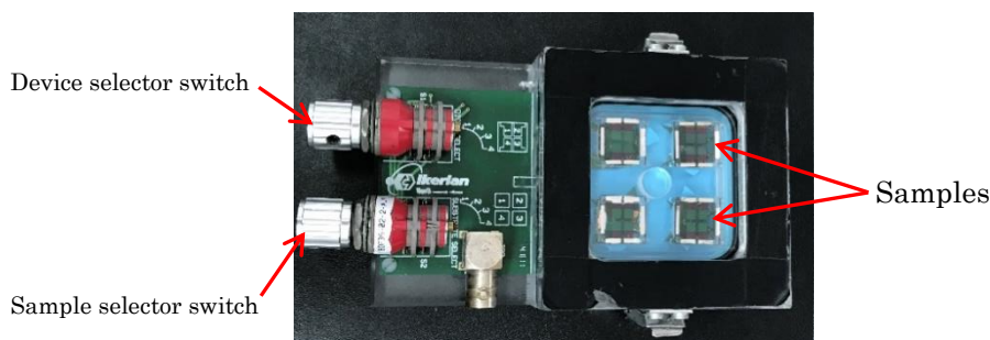
Figure 3.8 Samples-holder used for the transporting and characterization measurements of devices
