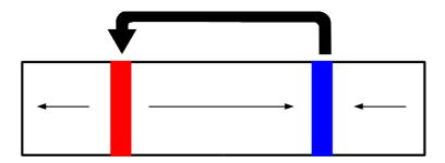
Figure 2.1: Schematic view of a NEMD simulation. The thick arrow represents that an amount of energy is extracted from the blue region and added to the red region after each step of the algorithm. This cools down the blue region and warms up the red, so in the natural evolution of the system there will be a heat flux going from the hot region to the cold region, represented in the image by the thin arrows.
