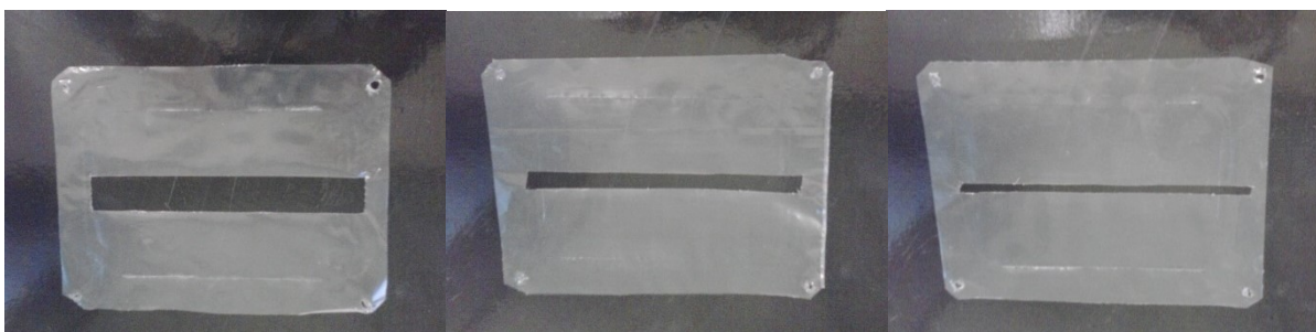
Fig. 2. Photograph of the plastic sheets used to block the membrane for each strip width: a) 2 cm, b) 1 cm, and c) 0.5 cm.
