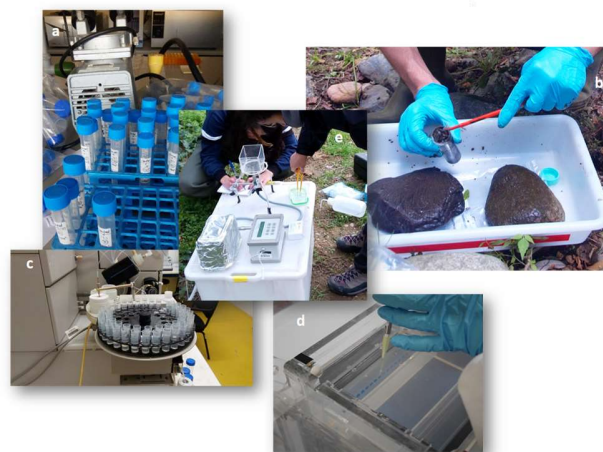
Figure 2. Images of some procedures followed to analyse water and biofilm samples. a) falcons for nutrient analysis, b) biofilm collection by scrapping, c) dissolved and bioaccumulated metal analysis, d) PCR products on agarose gel, e) Chl-a fluorescence measurements. From María Argudo and Helena Guasch.
