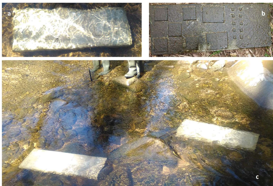
Figure 1. Set up of biomonitoring study with biofilm. a) Artificial substrate before biofilm colonization, b) and after seven weeks of colonization, c) Artificial substrata on the streambed. From Carmen Espinosa and María Argudo.
