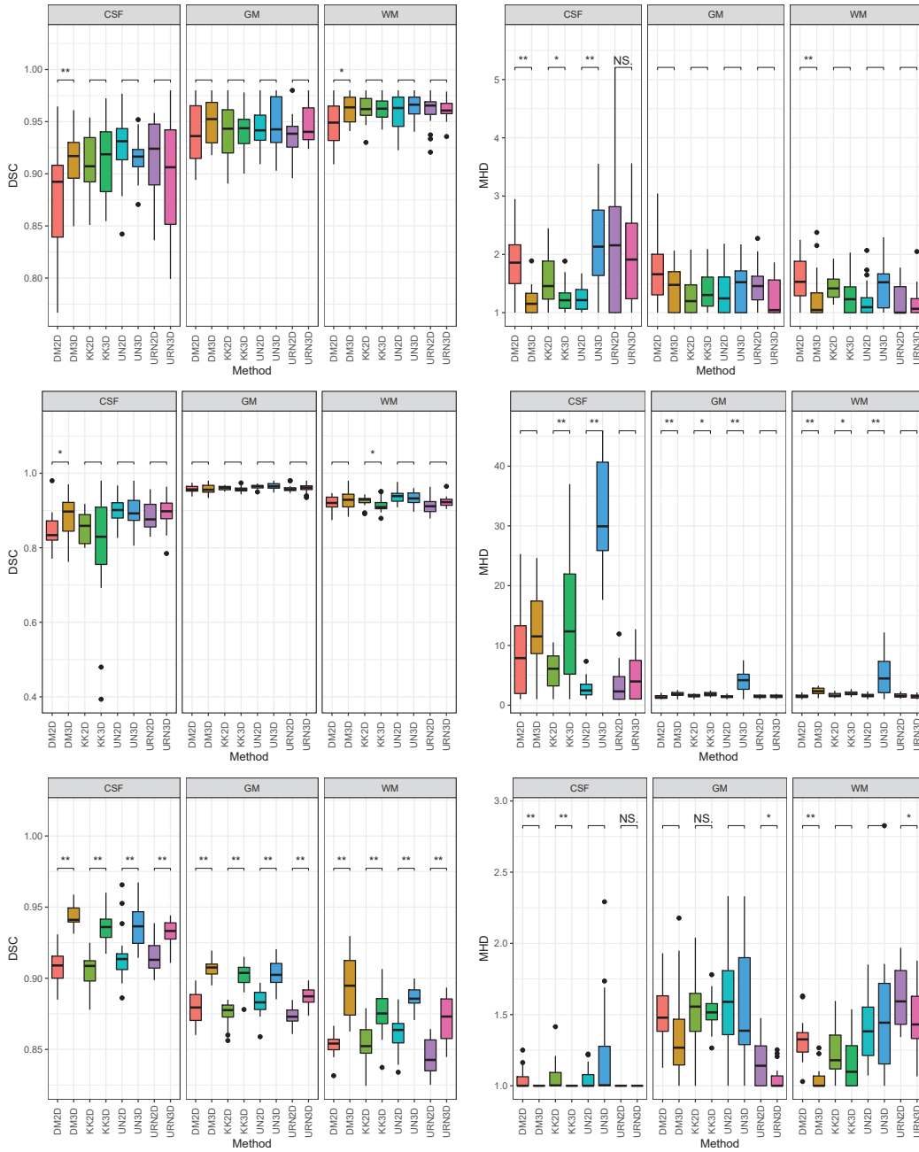
Figure 4.7: DSC (left column) and MHD (right column) values obtained using 2D and 3D versions of the same architecture. From top to bottom, boxplots for MICCAI2012, IBSR18, and iSeg2017, respectively. DM, KK, UN, and URN refer to the networks inspired by the works of Dolz et al. [103], Kamnitsas et al. [152], Çiçek et al. [148], Guerrero et al. [159], respectively. The subindex indicates the network dimensionality. Differences between both versions of the same baseline architecture are highlighted with NS, *, and ** indicating a p -value > 0.1 , < 0.05 and < 0.01 , respectively. CSF: cerebrospinal fluid. GM: grey matter. WM: white matter.
