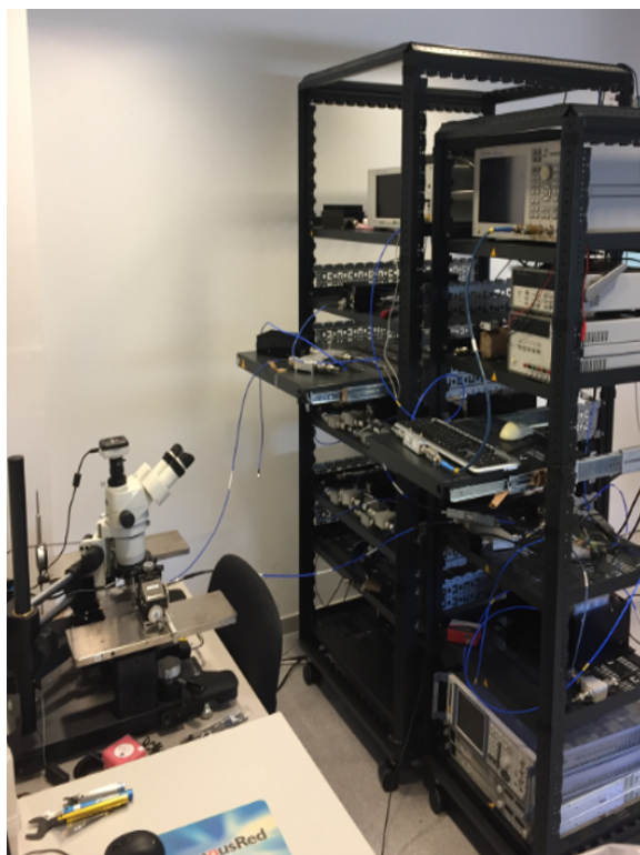
Figure 4.9: IMD3 measurement system configuration in the UPC RF laboratory, CSC-EETAC.
