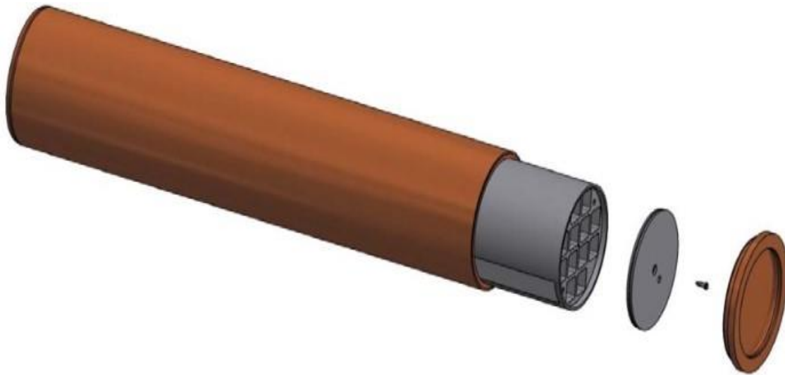
Figure 1-2 Canister components (Jonsson et al., 2018).
