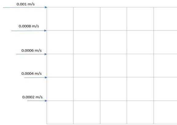
Figure 3-6 Different displacement rates are used in a simple shear test in the X-direction.
